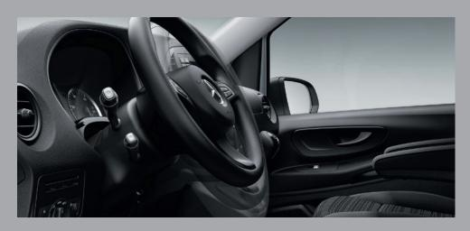
The steering wheel is adjustable for reach and rake to allow drivers of different sizes to adopt an individual, ergonomic posture.
