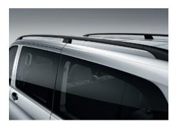
The roof rails allow bulky items to be transported on the vehicle roof and enhance the look of the vehicle.
