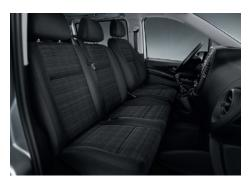
• The **twin co-driver seat** with adjustable headrests and 3-point seat belts offers space for two co-drivers.
