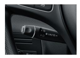
Cruise control helps to maintain a set speed, making the driver's job easier. SPEEDTRONIC speed limiter also makes it easier to maintain a set speed, for example in motorway road works
