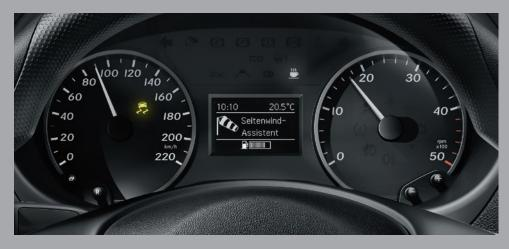
The standard-fit Crosswind Assist helps to prevent lateral drift of the vehicle due to gusting crosswinds.
