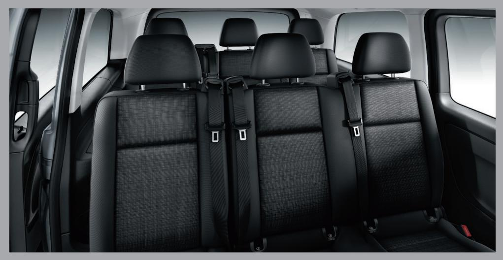
The passenger compartment of the Vito Tourer PRO offers space for seven passengers as standard. The outer seat has an EASY-ENTRY function, allowing comfortable through-access to the second seat row. If required, this seat can be completely removed. All seats are fitted with integral 3-point seat belts and height-adjustable headrests. Child seats with ISOFIX attachment points can be fitted to all seats.
