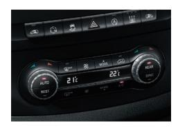
• THERMOTRONIC regulates the temperature, airflow and air distribution separately for the driver and co-driver.
