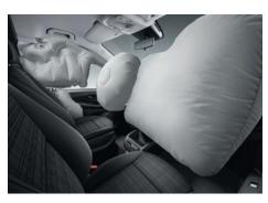
The airbags for the driver and co-driver and thorax/ pelvis sidebags and windowbags in the front form part of the standard safety equipment.
