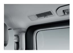
TEMPMATIC semi-automatic climate control in the rear optimises ventilation in the passenger compartment with evenly distributed warm or cool air.
