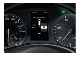
Active Parking Assist helps the driver find somewhere to park and assists when reversing into or out of a parking space.
