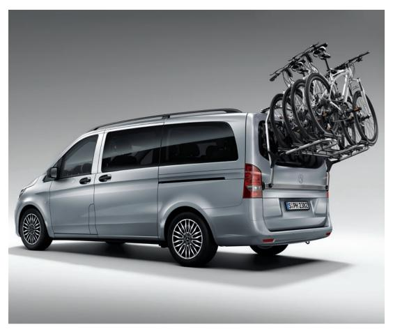
Rear-mounted bicycle rack, on tailgate. Easy-to use, lockable rear-mounted bicycle rack, designed to provide secure transport for 2 or 3 cycles. Rack is easy to attach to trailer coupling, and cycles are equally easy to fit to rack. Maximum payload of up to 30kg per rail, making rack suitable for most bikes.
