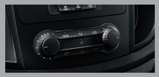
TEMPMATIC automatic temperature control regulates the desired temperature for the driver and front passenger.
