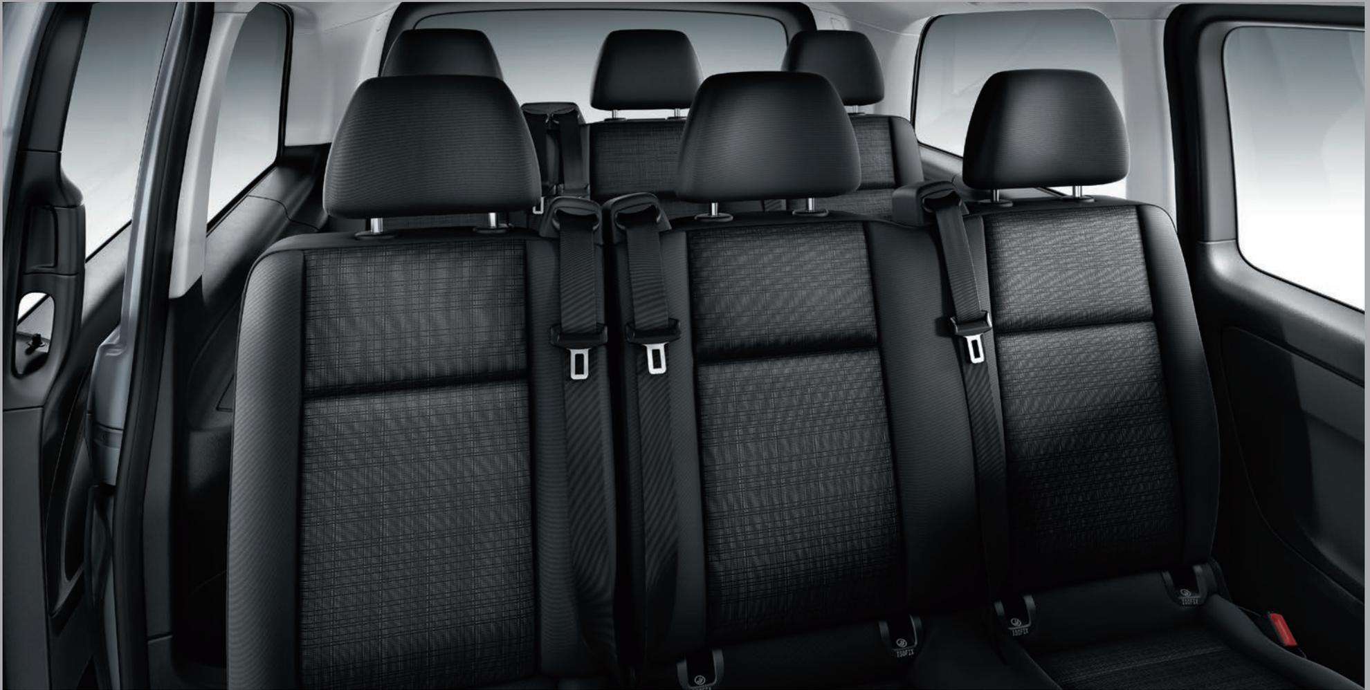
The passenger compartment of the Vito Tourer PRO offers space for seven passengers as standard. The outer seat has an EASY-ENTRY function, allowing comfortable through-access to the second seat row. If required, this seat can be completely removed. All seats are fitted with integral 3-point seat belts and height-adjustable headrests. Child seats with ISOFIX attachment points can be fitted to all seats.
