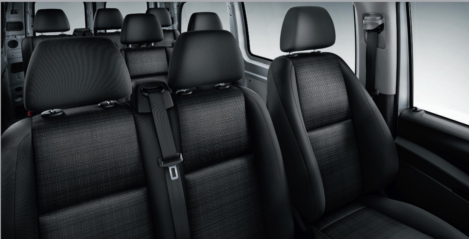
The passenger compartment of the Vito Tourer can be configured according to requirements: for example with a 2-seater bench in the first row and a 3-seater bench in the second. The 2-seater bench allows generous through-access to the rear. All seats are fitted with integral 3-point seat belts and height-adjustable headrests. Child seats with ISOFIX attachment points can be fitted to up to four seats.
