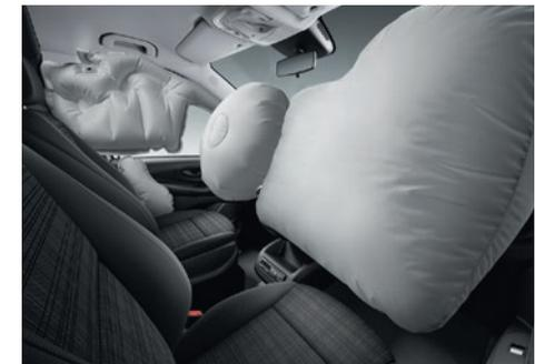
● The **airbags** for the driver and co-driver and thorax/pelvis sidebags and windowbags in the front form part of the standard safety equipment.
