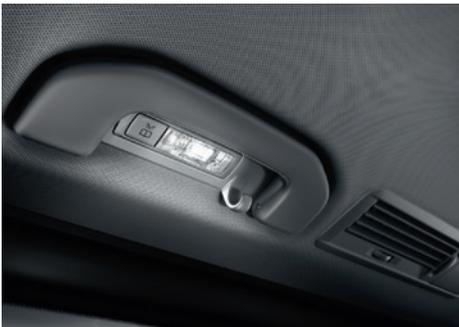
○ The **interior and ambient lighting function** enhances comfort. It includes the reading light in the grab handle as well as courtesy lights.<sup>1</sup>
