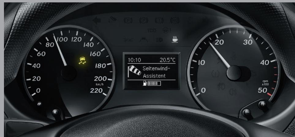
The standard-fit Crosswind Assist helps to prevent lateral drift of the vehicle due to gusting crosswinds.
