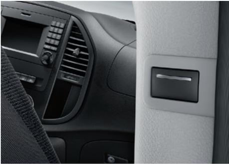
○ The **electrically operated sliding doors** can be opened and closed at the touch of a button.
